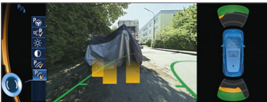
Rear view camera, view in CID with parking assistance lines and obstruction marking
